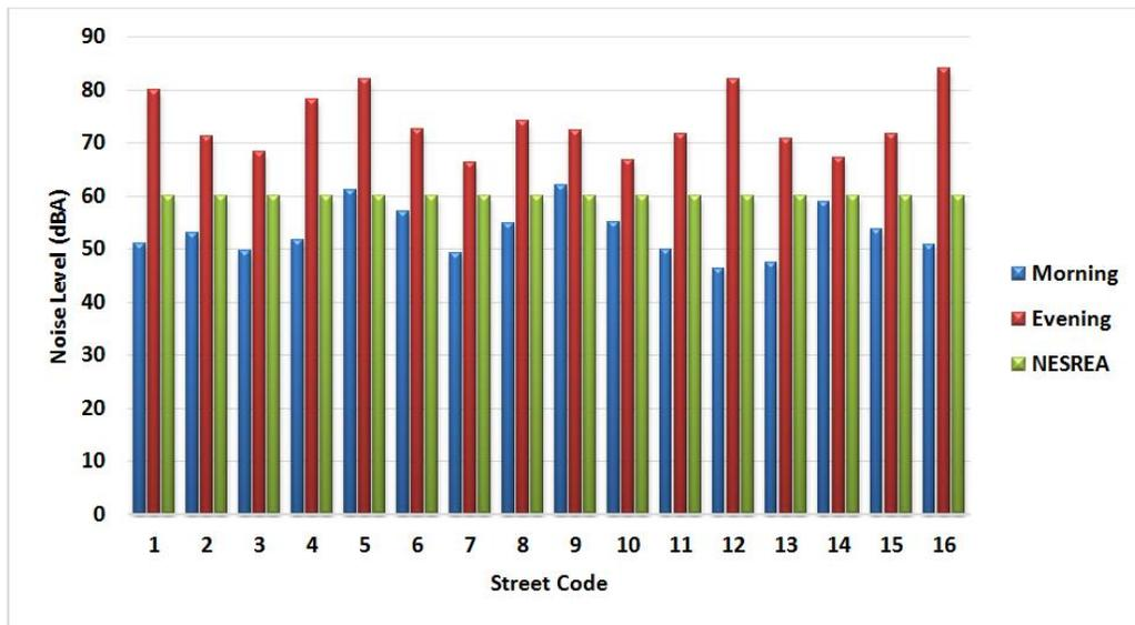
**Fig. 4. Comparison of Noise Levels [dBA] from power-generating sets in Nnewi North with NESREA permissible limit**
